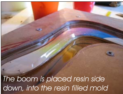
The resin is topped up to the centerline
