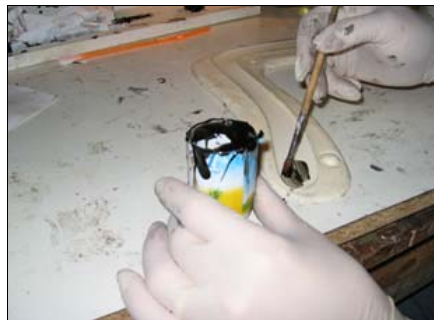
Painting on the Gel, to the mold surface.
