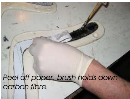
The uni tape goes in from the elbow to the tip
