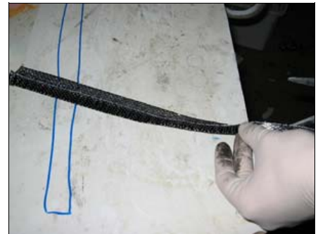
Tape is folded in to its centre
