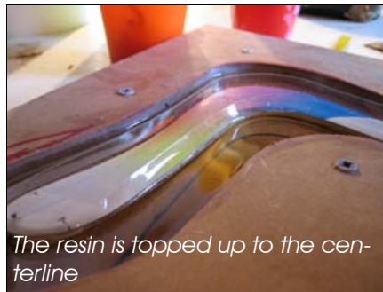
Mark out where more resin is needed
