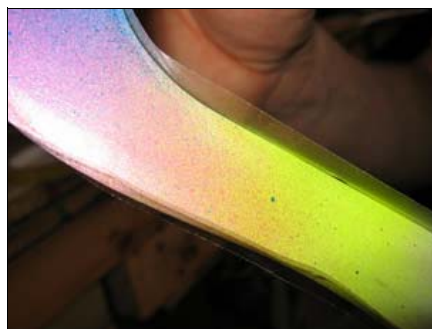
Sellotape the edge of the boomerang, all the way round.
