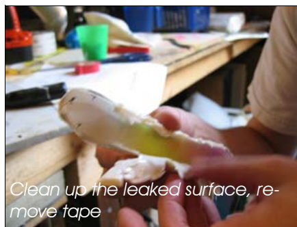
After the first pour (yes its leaking!)
