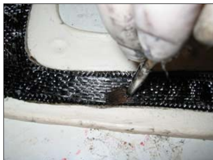
Dabbing vinyl onto the uni tape
