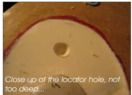
Drill the locator holes
