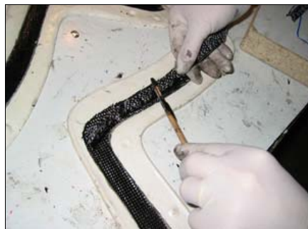
The uni tape goes in from the elbow to the tip
