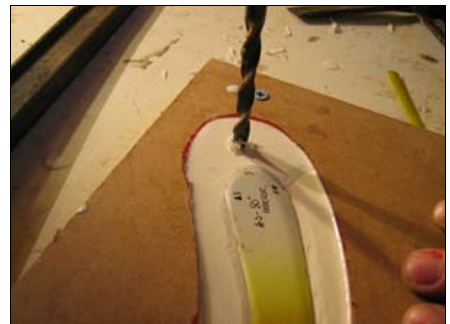
Drill the locator holes
