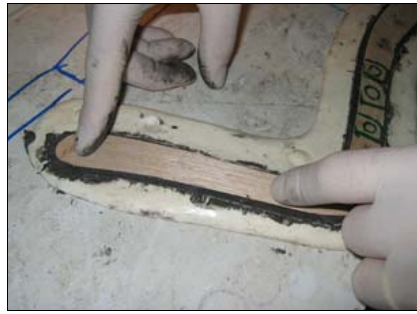
Lay the balsa down
