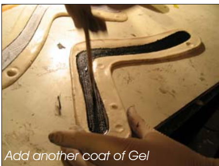
Dabbing vinyl onto the uni tape
