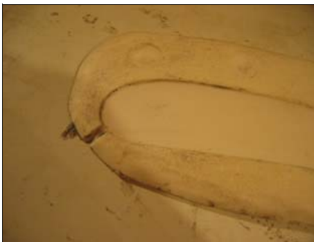
The grooves let out resin during clamping
