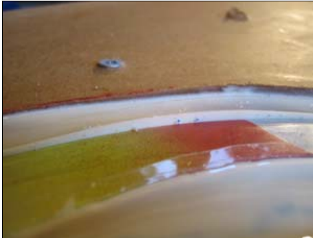
Here you can clearly see where too much resin sets on the tape - it should ideally be up to the center-line only
