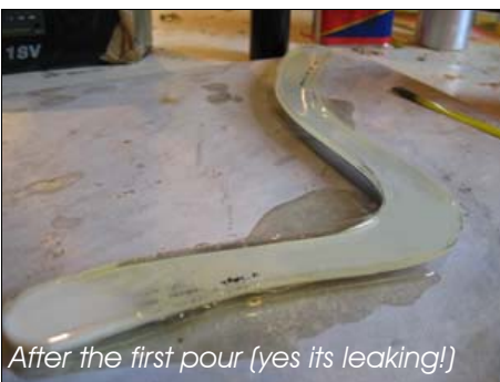
Clean up the leaked surface, remove tape
