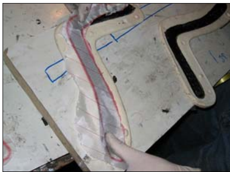
Peel ply onto the wet carbon fibre
