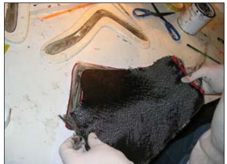
Lay the carbon onto the gel paper
