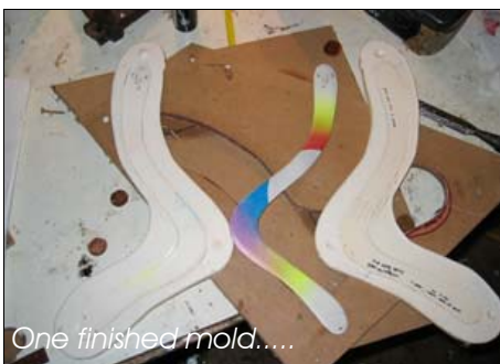
The grooves let out resin during clamping
