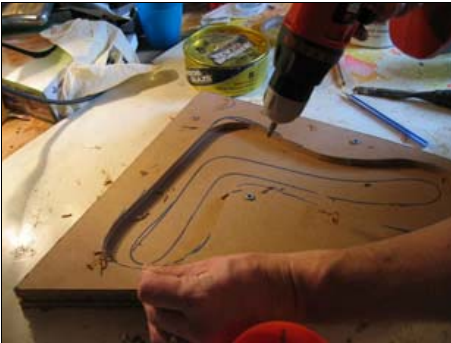
Join upper and lower sections after cutting.
